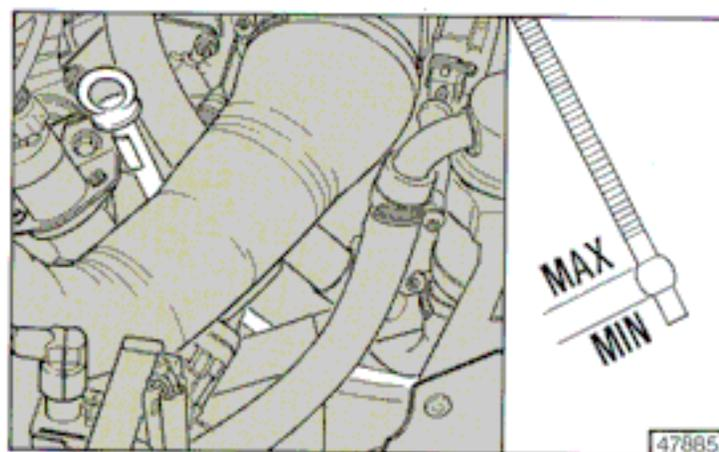
When the level is near or below MIN, top up through the dipstick housing until reaching MAX.
